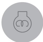
This lamp comes on when the glow plugs (if fitted) are activated.
