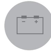
This warning lamp comes on when the system voltage is connected.
