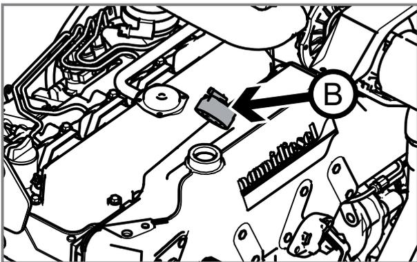
1. Turn the coolant filler cap **B** slowly to the first stop and let any pressure escape from the system then remove the cap.
