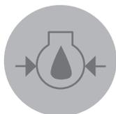
This warning lamp lights up and the alarm sounds when the engine oil pressure is too low.
