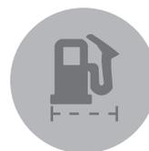
This lamp lights up and the alarm sounds when there is too much water in the fuel filter of the engine (not applicable on some engines).
