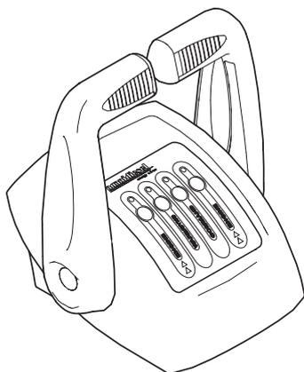
On most boats, the control lever controls both the engine rpm and the gear shift (ahead / astern). However, some boats can be equipped with a separated shift command.
