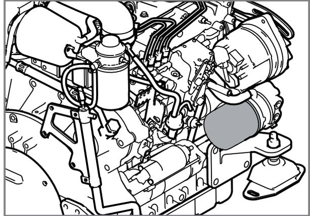
1. Remove the oil filter with a filter wrench. Turn the filter counter-clockwise. Remove the gasket.
