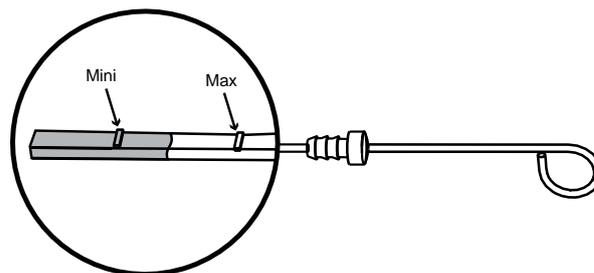
If the level is too low, remove the oil filler plug and add oil slowly. Wait few minutes before checking the oil level to let the oil drain down to the oil pan.
