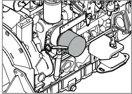
1. Remove the oil filter with a filter wrench tool. Turn the filter counter-clockwise (CCW). Remove the gasket.
