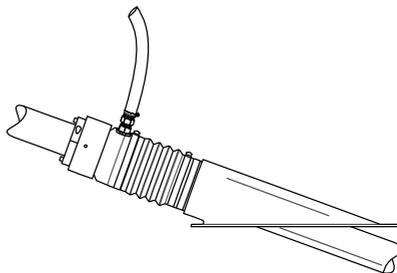
If the boat is equipped with a braided-type stuffing box, check the system's tightness. As this system is not absolutely tight, it is normal that a slight amount of water passes through the stuffing box. Correct operation is characterized by a drop-by-drop water intake. If too much water comes in, stop the engine and contact your Nanni dealer as soon as possible.
