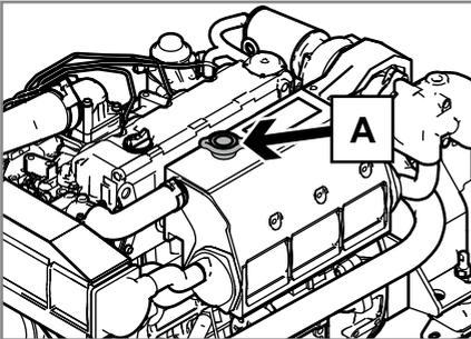
3. Coolant level should lie between the filler neck lower edge and the level spur.
