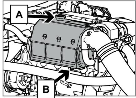
3. Drain off all coolant. Empty the recovery container as well as the hoses used in the process.
