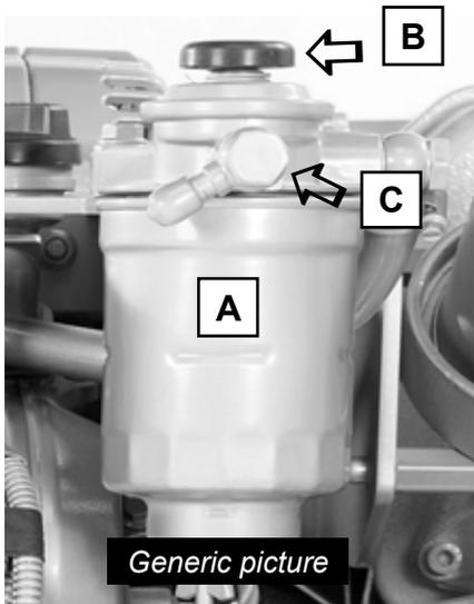
1. Close the fuel cock. Wipe up the holding filter bracket with a clean non flint cloth.
