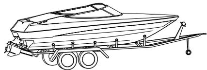
Before removing the boat out of water, raise the drive in the lift range and lock the transmission using the optional kit or any equivalent system. Put the drive in the lift range and lock the transmission using the optional kit or any equivalent system.
